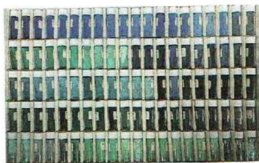
Fig. 3 Variation of colors of azurite and malachite (depending on particle size, degree of calcination and mixture of color) produced by Kiya
